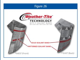
Mystique 42, Vangard 42 IR and Manoir laminate shingles have 2 sealant bands located on the front of the shingle as well as 2 release tapes (to prevent sticking during stacking) on the back which should not be removed (see Figure 27a).
